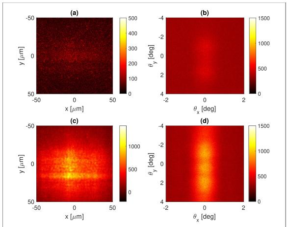
**Figure 3.** Illustration of the source plane (a) and (c) and far-field (b) and (d) intensity distributions. The pump-power for (a) and (b) is 275  $\mu$ J cm<sup>-2</sup>, and for (c) and (d) is 625  $\mu$ J cm<sup>-2</sup>. Measured parameters (a):  $w_x = 48.63 \ \mu\text{m}$ ,  $w_y = 39.98 \ \mu\text{m}$ , (b):  $\Theta_x = 0.93^\circ$ ,  $\Theta_y = 4.11^\circ$ , (c):  $w_x = 43.20 \ \mu\text{m}$ ,  $w_y = 43.00 \ \mu\text{m}$ , (d):  $\Theta_x = 0.79^\circ$ ,  $\Theta_y = 3.55^\circ$ .
