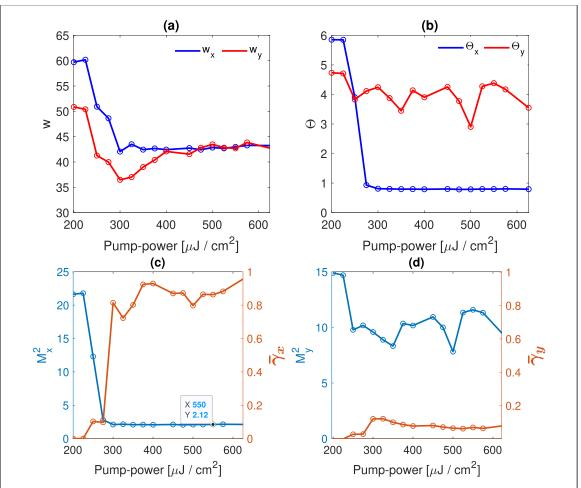
**Figure 6.** Evolution of the measured beam radii as a function of pump power. (a) The source plane beam widths, and (b) the far-field angular widths of the PLL radiation. (c)  $M_x^2$ , and (d)  $M_y^2$  superposed with the effective degree of coherence as a function of pump power. Blue:  $M^2$  values, orange: overall degrees of coherence.
